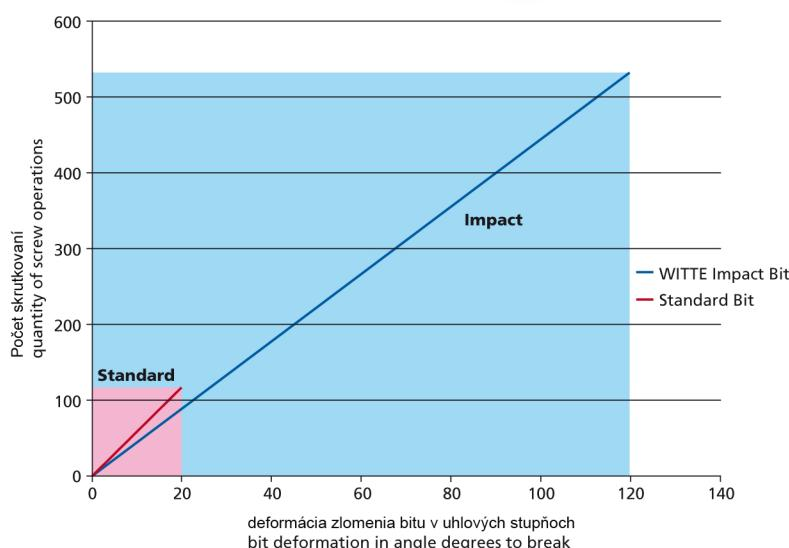
Professional cordless impact screwdrivers are more efficient and require special bits.
