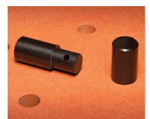
Removing the pins enables the dogs to insert into the HDF valchromat top with 20mm holes, code 102537
