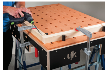
Using dogs and clamps to ensure the work piece is clamped square and level
