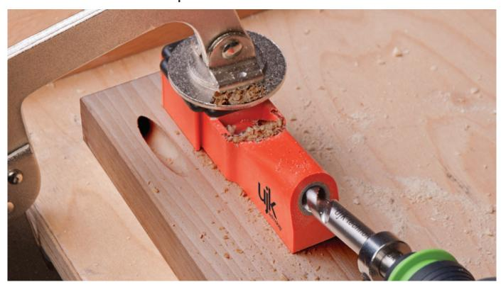
**Image 9** Finished drilled piece ready for the pocket hole screws.
