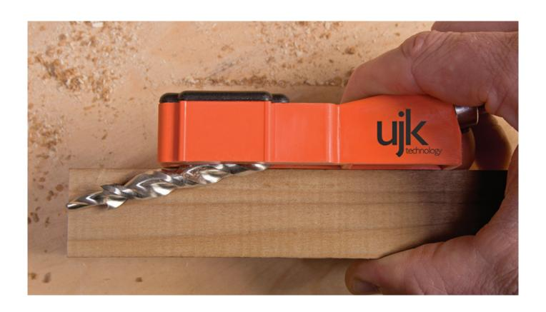
**Image 4** Lock the drill depth collar.
