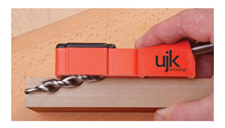
**Image 2** If using thinner material move the jig forward.
