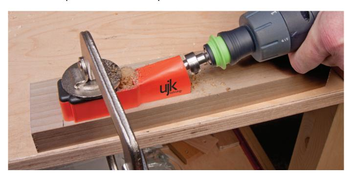
**Image 7** If your clamp doesn't have enough capacity an additional clamp will be needed.
