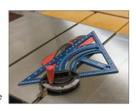
wider than the core. Loosen your miter gauge angle adjustment and slide it into your miter channel, up to the edge of the triangle as shown in the picture above. To calibrate your miter gauge at a perfect 90 degrees to your table saw blade, follow the same procedure but use the two shorter ends of the triangle.
